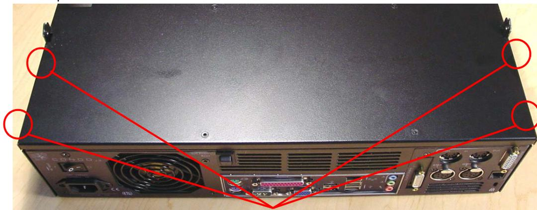
**Remove these screws (located on the side of chassis)**
